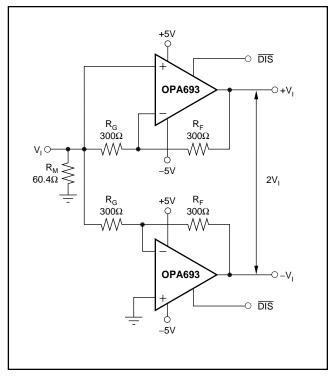
Figure 9. DC  $\rightarrow$  700MHz, Single-to-Differential Conversion.
