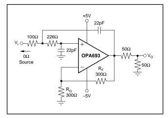
Figure 10. Line Driver with 40 MHz Low-Pass Active Filter.
