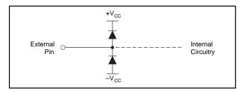
Figure 16. Internal ESD Protection.
