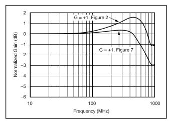
Figure 8. Buffer Frequency Response Comparison.
