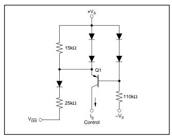
Figure 15. Simplified Disable Control Circuit.
