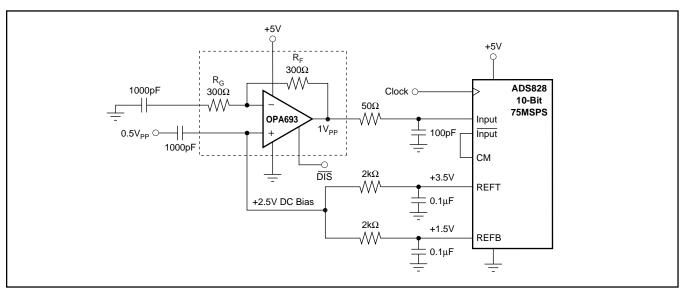
Figure 6. Wideband, AC-Coupled, Single-Supply ADC Driver.
