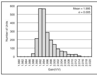
Figure 12. Typical +2V/V Gain Distribution.
