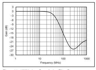
Figure 11. 40MHz Low-Pass Active Filter Response.
