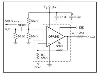
Figure 5. AC-Coupled, G = +1V/V, Single-Supply Specification and Test Circuit.
