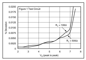
Figure 13. DC Linearity vs Output Swing and Loads.
